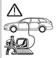
Match the vehicle code in the following control units via selected diagnostics by coding "towing hitch installed" (see coding example on page 13):
