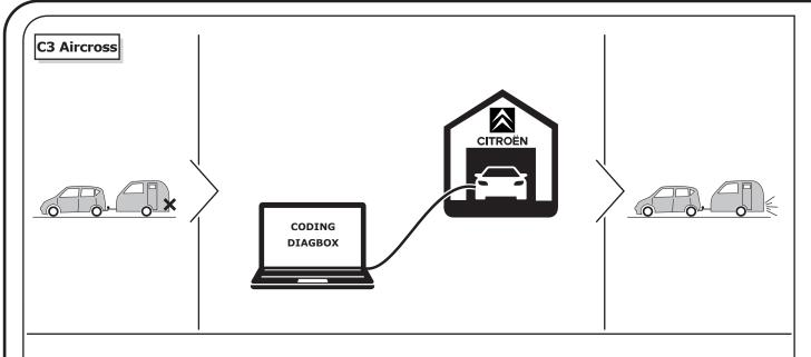
The activation of the trailer functions has to be carried out using the CITROËN DIAGBOX as follows:
