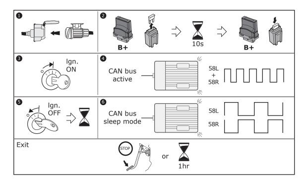
The faultless connection of the trailer module to the vehicle-side CAN-bus can be checked quick and easy with the ECS CAN-check:
