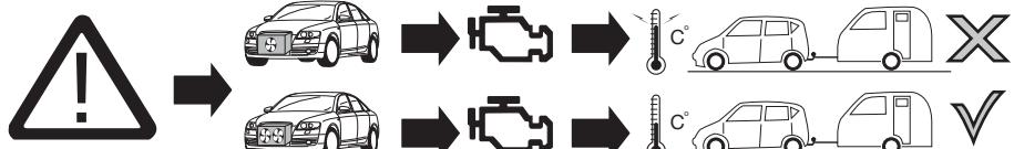
**ATTENTION!** The vehicle's cooling capacity may have to be increased when retrofitting a trailer coupling!
