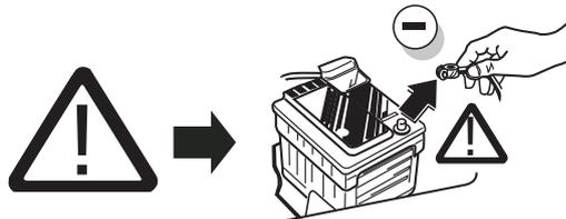
Note: It may be necessary to check if this vehicle has a stored radio code before disconnecting the battery!
