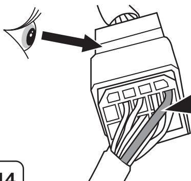
Please check if **B+/30** permanent power wire in trailer preparation connector has got a minimum diameter of **1,5 mm<sup>2</sup>**, if not please continue with **Option 2!**
