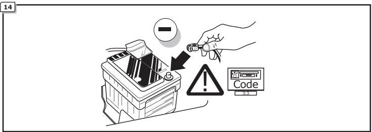
TEST ALL THE CIRCUITS WITH A TEST DEVICE WITH THE CORRECT POWER LOAD FOR EACH FUNCTION. A TEST DEVICE WITH LED'S CANNOT BE USED FOR THIS PURPOSE.
