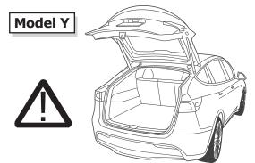
Please note that the operation of the automatic electric tailgate will continue to function with a connected bicycle carrier/trailer/caravan. It must be operated manually.
