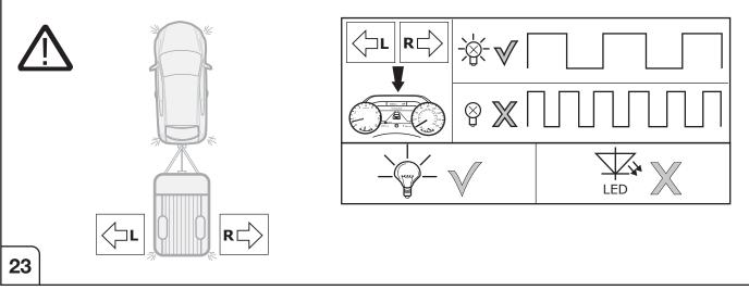
The following lamp functions for the trailer are not supported by all towing vehicles with DRL circuit:
