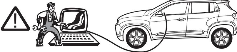
The light functions on the trailer will only operate **AFTER** the vehicle has been re-coded!
