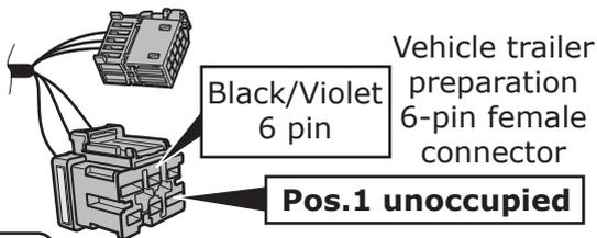
Vehicle trailer preparation 6-pin female connector
