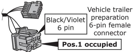
Vehicle trailer preparation 6-pin female connector
