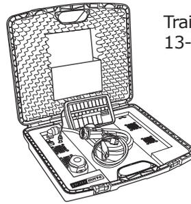
Trailer Simulator for 7- and 13-pin Sockets
