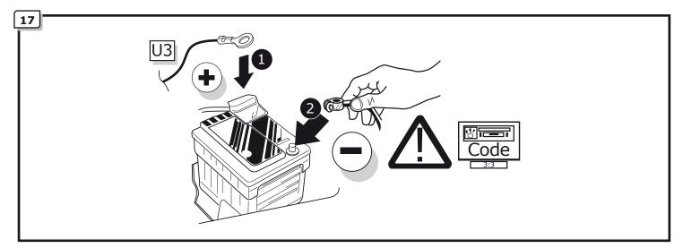
TEST ALL THE CIRCUITS WITH A TEST DEVICE WITH THE CORRECT POWER LOAD FOR EACH FUNCTION. A TEST DEVICE WITH LED'S CANNOT BE USED FOR
