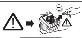
Note: It may be necessary to check if this vehicle has a stored radio code before disconnecting the battery!
